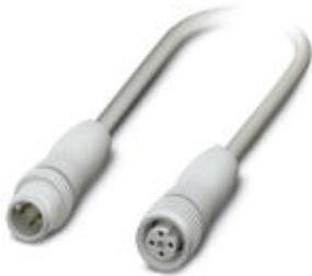
Sensor/Actuator cable, 4-position, PP-EPDM halogen-free, Gray RAL 7035, Plug straight M12, A-coded, on Socket straight M12, A-coded, Cable length: 1.5 m, Hygienic design, with plastic knurl
